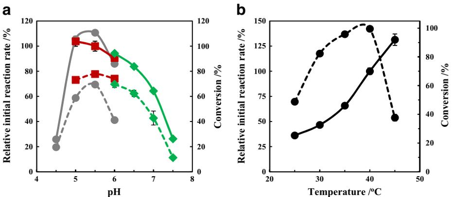
**Fig. 4** Effect of reaction buffers and temperatures on the decarboxylation of tyrosine catalyzed by TDC. **a** Reaction buffer: (●) NaAc-HAc buffer, (■) Na<sub>2</sub>HPO<sub>4</sub>-KH<sub>2</sub>PO<sub>4</sub> buffer, (◆) K<sub>2</sub>HPO<sub>4</sub>-KH<sub>2</sub>PO<sub>4</sub> buffer, (dotted line) conversion ratio, (solid line) relative initial reaction rate. **b** Temperature: (dotted line) conversion rate, (solid line) relative initial reaction rate
