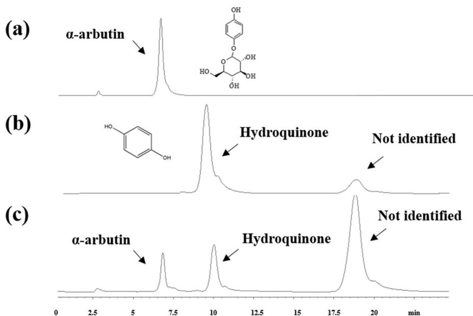
Fig. 6. HPLC chromatogram of transfer reaction of hydroquinone by *TtSPase*. (a) The standard of α-arbutin. (b) Substrate of hydroquinone. (c) Reaction mixture by *TtSPase*.
