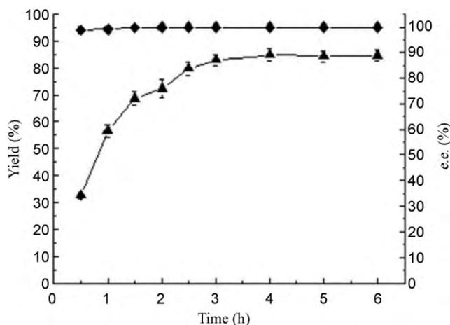
**Fig. 6.** The time courses of the enzymatic reduction of OPBE in aqueous medium. (▲) Yield. (◆) *e.e.* value. Reaction conditions: 10 mM OPBE, 10 mM NADPH, and approximate 0.2 U of purified enzyme in phosphate buffer (100 mM, pH 6.0) at 30 °C (200 rpm) for 6 h.
